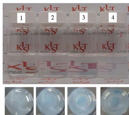
Figure 6. Dispersability of zinc oxide nanoparticles in ethylene glycol. The zinc oxide particles were synthesized using (1) \text{scH}_2\text{O} , (2) \text{scMeOH} , (3) \text{scMeOH} with 0.05 M \text{Zn}(\text{NO}_3)_2 and 0.3 M decanoic acid, (4) \text{scMeOH} with 0.01 M \text{Zn}(\text{NO}_3)_2 and 0.3 M decanoic acid. The bottom pictures were the bottom view of the vials.
